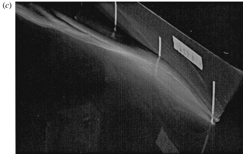
FIGURE 5. The wave structure around the ship at Fr_L = 0.334 : (a) side view; (b) top view; (c) the liquid film around the bow.
